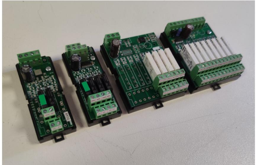
The XRD2 / 4/8 module is a driver with 2/4/8 low current 0-10V analog inputs, which allows you to activate two, four or eight relay outputs with voltages from 1.5 V. Each relay output has of a NO contact (option -S, SPST) or NO / NC (option -D SPDT) and LED status indicator. It comes mounted on a DIN rail module, extra flat without cover.
