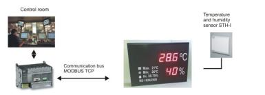
**MTH-EA** allows to connect two external analog inputs for temperature and humidity. Includes power cord.
